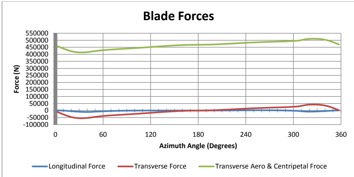
Figure 34 – Forces Acting on Turbine Blade Over One Rotation
