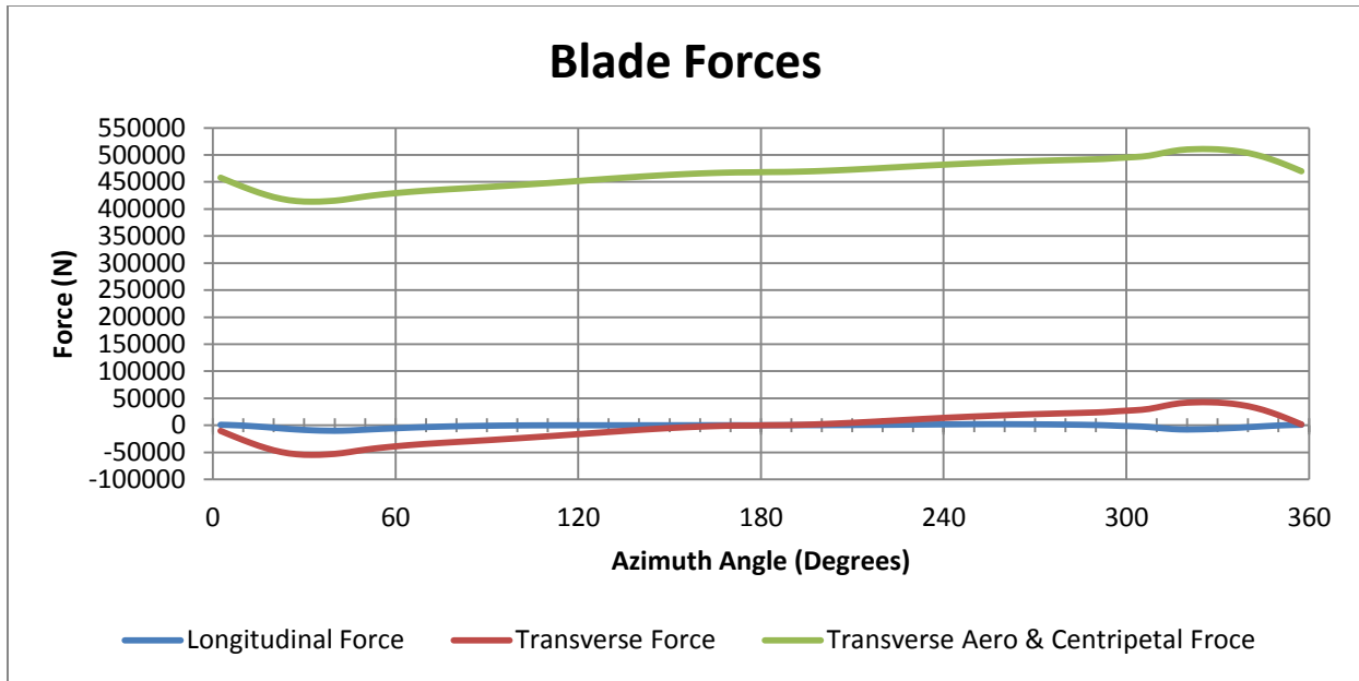
Figure 26: Blade forces from aerodynamic analysis and centripetal force calculations
