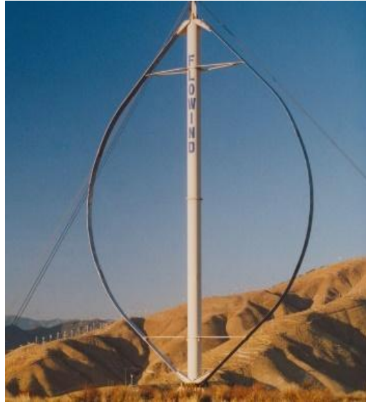
Figure 2: FloWind Full-Darrieus VAWT
